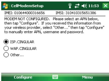
Depending on your wireless provider, there may only be one selection. Select one of the choices presented on this screen and tap on the *Configure* button at the bottom of the screen. The handheld performs a reset to configure the modem with these settings.
