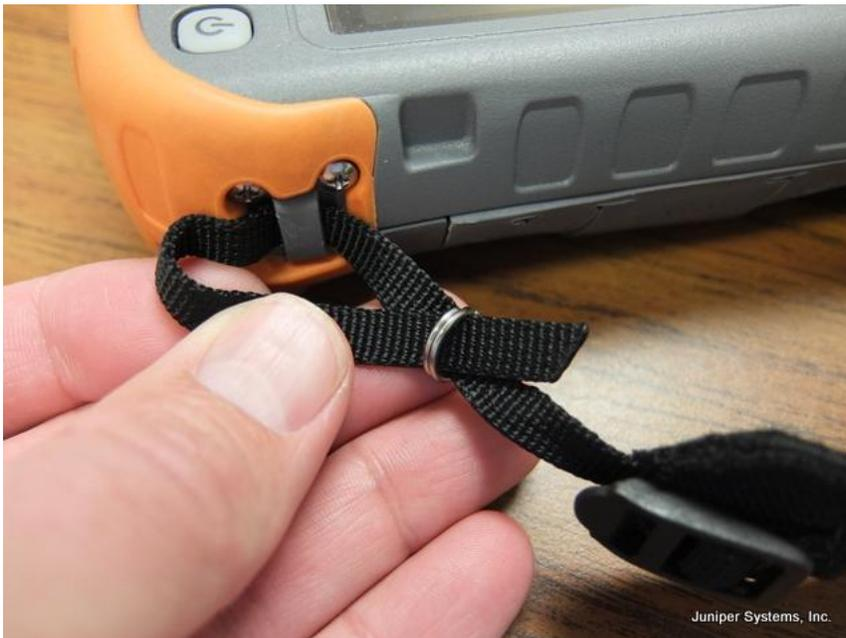
Attach the hand strap tether end to the hand strap buckle.
