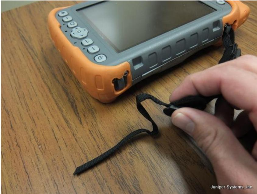
Slide one of the rings onto the hand strap tether.
