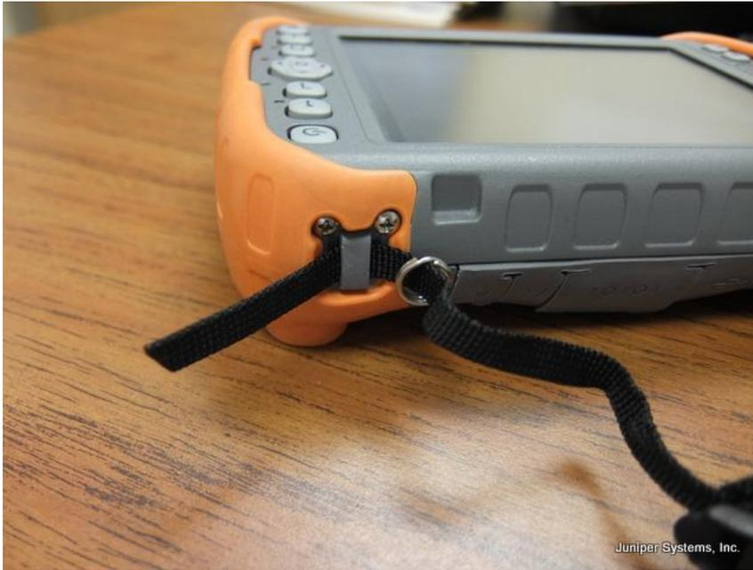
Slide the hand strap tether end back through the ring.
