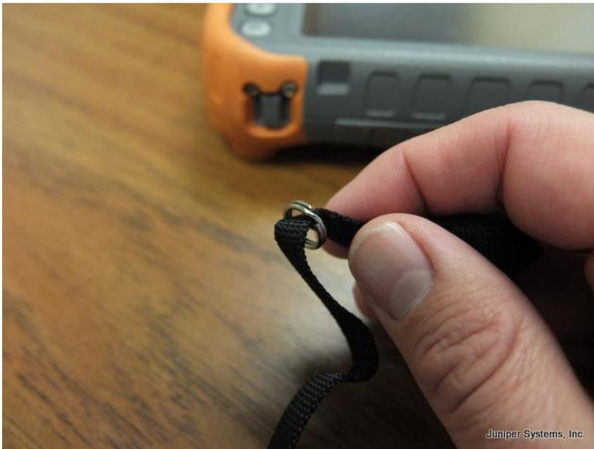
Slide the hand strap tether through the attachment loop on the Mesa.
