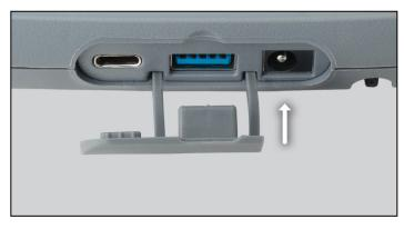
4. Insert the stylus connector into the power input jack.
