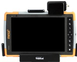
6. To remove the Mesa 2, turn the key until the lock button pops out. Lift the lock bar, and remove the Mesa 2.
