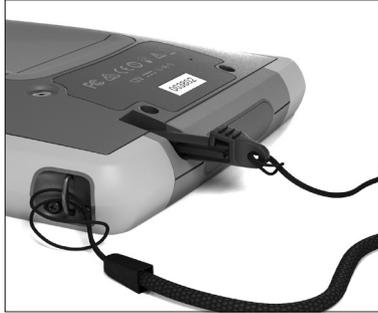
2. Insert the stylus with the attached tether through this loop and tighten the loop.
