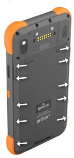
4. Slide the battery door locks into the locked position.
