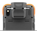
5. Route the hand strap through the hand strap mounting loop at the bottom of the barcode scanner expansion, if desired.
