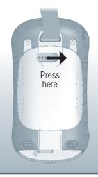
1b. Press on the battery door and slide the latch to the right.
