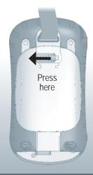
1f. Press on the battery door. Slide the latch to the left to lock it.
