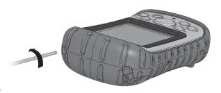
2. Insert your card. To keep your card securely in its slot, cushion it by placing small or mediumsized foam pieces inside the top of the cap. Insert enough foam into the cap so that when you slide the cap back onto the Field PC with little pressure, a ¼ inch (6 mm) gap remains between the cap and the Field PC as shown.
