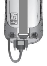
Make sure the seal adapter plate is properly installed.
