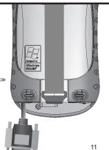
**4.** Connect the sensor connector to the 9-pin serial port or USB host port.
