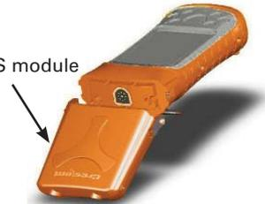
6. Align GPS module with the interface module.
