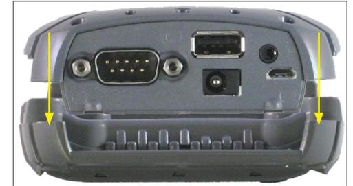
4. Firmly press on the board above the pins, *not* on the plastic. Press until the pins seat in the connector and there is no gap between the module and the unit.
