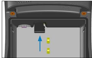
5. Replace the battery pack, and attach the battery door.
