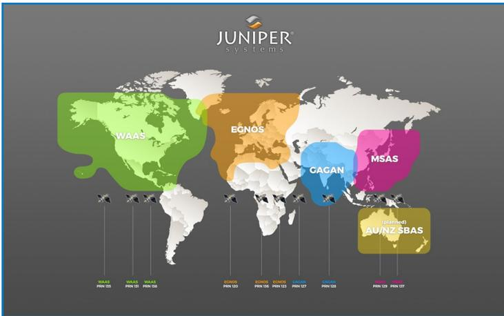
For example, if you are collecting corrected GPS positions in the Northeastern United States, the Archer 3 may be receiving SBAS corrections from WAAS or EGNOS. If the receiver is set to Auto, it may even jump back and forth between the two. The two services use different reference datum or models. Switching between them can cause significant error between different points of data.
