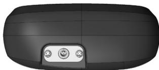
When an external GNSS antenna is attached, the GNSS receiver will automatically detect and use the external antenna. Otherwise, the GNSS receiver will use the internal GNSS antenna.
