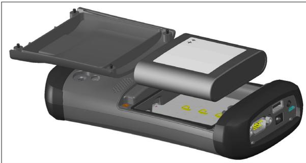
2. If you are using a micro SD card for additional memory or a SIM card with the 3G Data Modem (optional), you can install them now before you install the battery pack
