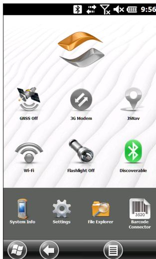
If the *Bluetooth* gadget is not on your Home screen, you can get to the desired control panel by selecting *Getting Started* and either *Set up a Bluetooth device* or *Set up a Bluetooth COM Port*. You can also press *Start > Settings > Connections*.
