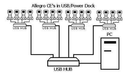
The USB/Power Docks can be connected to the hubs and PC in any order. There is no fixed connection pattern required.
