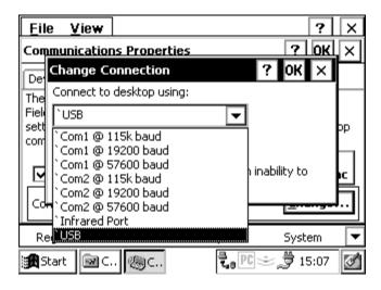
To connect remove the Allegro from the USB/Power Dock then place it back into the USB/Power Dock. This will automatically start the connection process.
