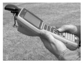
both TSIP and NMEA protocols with autonomous accuracy of 5–10 meters, or 2–5 meters after differential correction. The GPS expansion pod is used in conjunction with the following programs:
