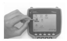
Three styli are provided: two small on-board stylus and a full size pen-type stylus. The small on-board stylus snaps into a holding bay built into the top of the Allegro. The Allegro can only hold one on-board stylus at a time. Other pointed objects can be used, including your finger. Be sure to use a device that will not scratch the screen.
