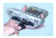
8) Charge the battery pack at room temperature until the charge indicator on the Allegro turns off. This can take 3 to 5 hours the first time you charge the battery.
