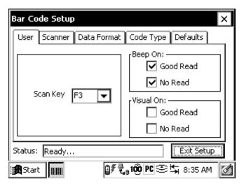
Only one Allegro key is used to both target and scan a bar code. Pressing on the scan key initiates the target beam first. The target beam stays on for a set time ranging from 0.0 to 9.9 seconds. You have the ability to set the target time, see later in this section. As soon as the target beam turns off, the scan beam turns on. The scan beam remains on until a valid scan is completed or until the maximum scan time is reached.
