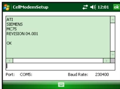
The current port is displayed along with the current baud rate. In this example, the Cellular Modem Expansion Pod has not yet been configured. **Port:** is “COM5.” When it is configured, **Port:** will be “VCA2.”
