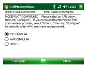
Depending on your wireless provider, there may only be one selection. Select one of the choices presented on this screen and tap on the *Configure* button at the bottom of the screen. The handheld performs a reset to configure the modem with the settings you selected.
