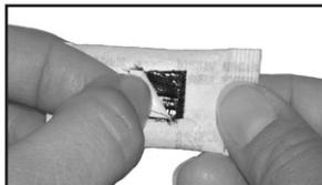
3. Attach the desiccant pack with the attached Velcro pieces so it is about  $\frac{1}{4}$  inch below the upper gasket rim and centered between the PC card door holder tabs. Make sure the lower edge of the desiccant pack sits directly above the PC Card holder tabs.
