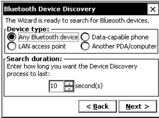
This screen enables you to limit the type of Bluetooth devices that the discovery process searches for. You can also specify the length of time the Allegro searches for devices. One of the following *Device types*: must be selected to proceed with the *Discovery Wizard*:
