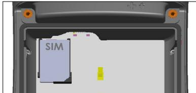
To remove the SIM card, pull the tray open and remove the card. Push the empty tray in until it catches.
