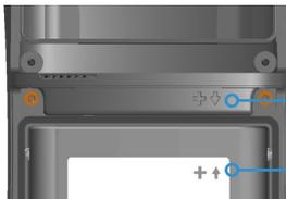
Line up the symbols on the case and the battery pack as shown
