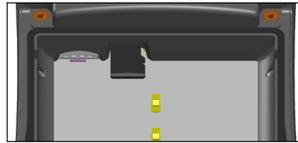
5. Replace the battery pack, and attach the battery door.
