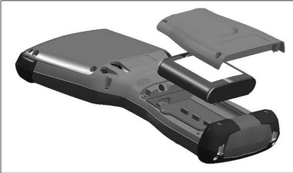
2. If you are using a micro SD card for additional memory or a mini SIM card with the 4G LTE (optional), you can install them now before you install the battery pack, or at another time. See more details about these cards later in this manual.
