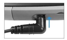
4. Loop the stylus cable around the hand strap to keep it from pulling free of the power input jack during use.
