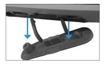
For other field computers, pull the connector cover down to access the power input jack.
