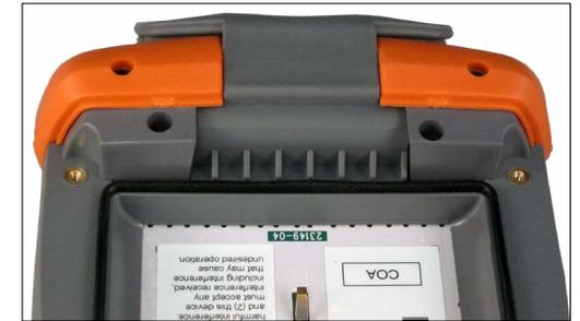
5. Place the Li-Ion battery pack in the compartment. Make sure the symbols on the battery pack label align with the symbols inside the compartment.
