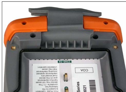
4. To install the new connector protector, insert the retention end into the area below the connector module. Press it under the battery door screw holes as shown.
