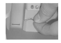
empty pin slot. 6. Reconnect the power and USB cables to the Power 3. Using your fingers, place the new pogo pin into the
