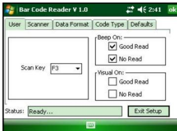
Only one Field PC key is used to both target and scan a bar code. Pressing on the scan key initiates the target beam first. The target beam stays on for a set time ranging from 0.0 to 9.9 seconds. You have the ability to set the target time, see *Scanner Setup*. As soon as the target beam turns off, the scan beam turns on. The scan beam remains on until a valid scan is completed or until the maximum scan time is reached.
