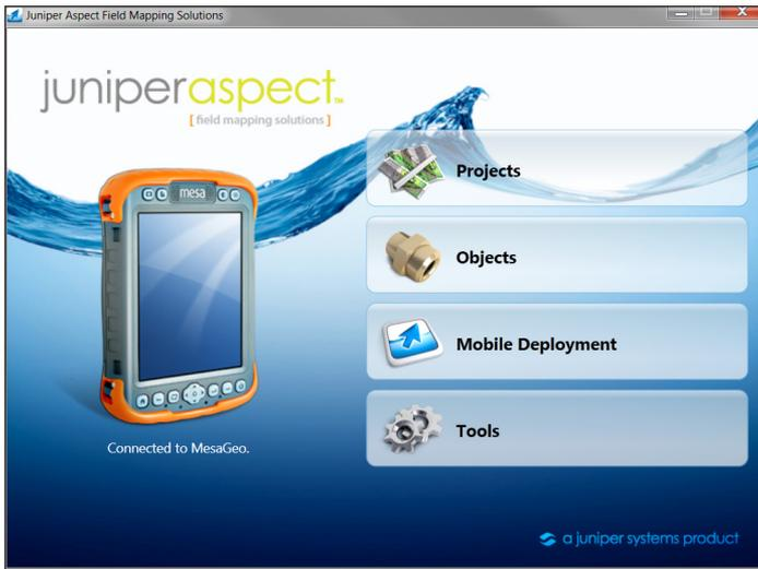
When the desktop computer and mobile computer are communicating with each other, the mobile computer graphic on the left side of the screen is shown with orange bumpers with the caption "Connected to (your device name)." If they are not communicating, the graphic is gray and the caption says "No Device Connected."
