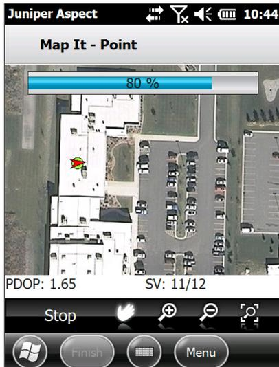
9. If you are mapping an object like a pipe or wire, you need to map two or more points to show where the pipe runs. Additional points for an object are mapped by selecting the capture button at the bottom of the screen. Each time you tap the capture button it will map another point, and you will see a progress bar while information is acquired from the GPS receiver.
