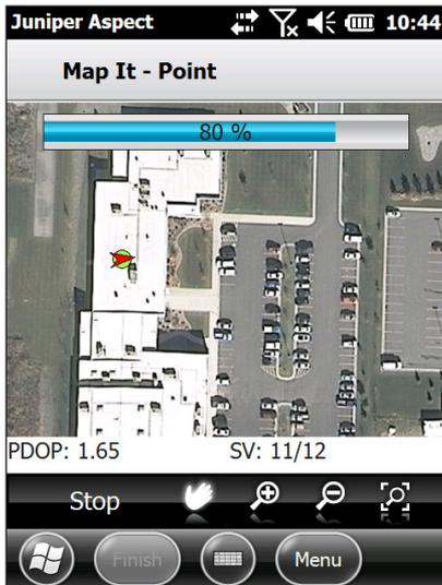
9. If you are mapping an object like a pipe or wire, you need to map two or more points to show where the pipe runs. Additional points for an object are mapped by selecting the capture button at the bottom of the screen. Each time you tap the capture button it will map another point, and you will see a progress bar while information is acquired from the GPS receiver.
